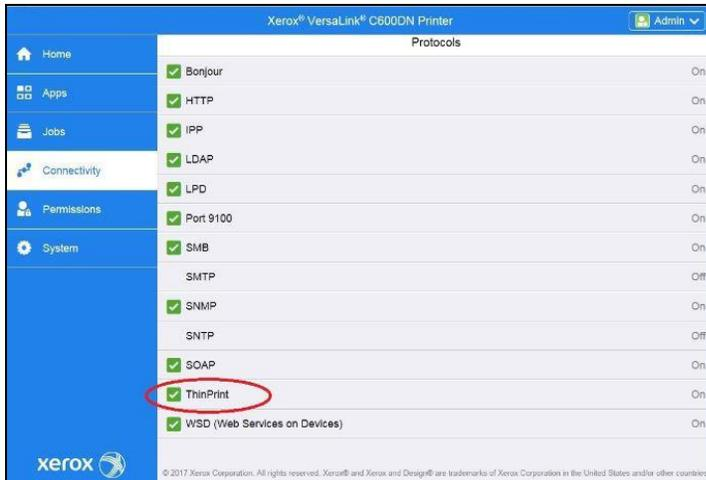
Once the ThinPrint Protocol is enabled the Admin has access to the settings below. The port must be enabled. The default port number for ThinPrint communication is 4000.
